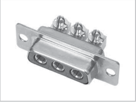
Fig. 3: Mixed Layout socket connector, contact arrangement 3W3, 3 high power contacts with right angled PCB termination in press-fit version
